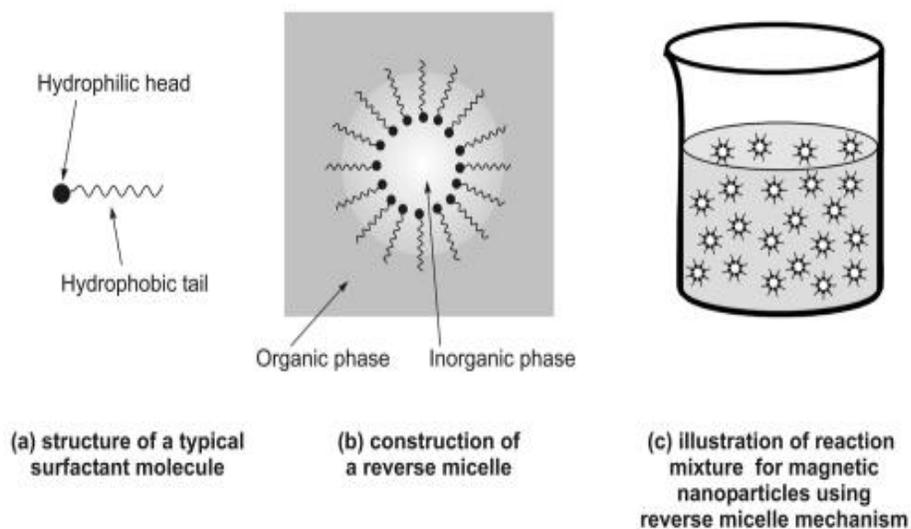
**Figure 1:** Schematic diagram of reverse micelle.
